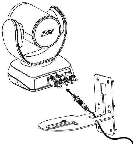
6. Use the remaining screws (included in package) to secure the camera on the L-mount bracket.
