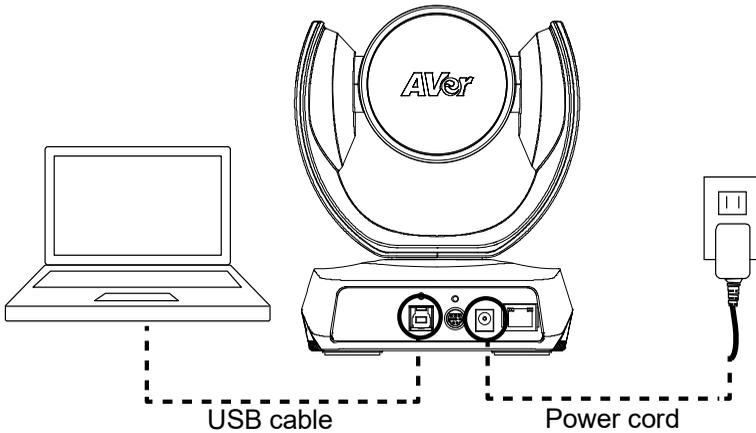
1. Use USB cable to connect the CAM520 Pro2 to your PC/laptop (refer to diagram above).
