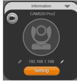
5. Set up IP address. The camera default IP address is **192.168.1.168**. Click pencil icon (✎) to edit IP address.
