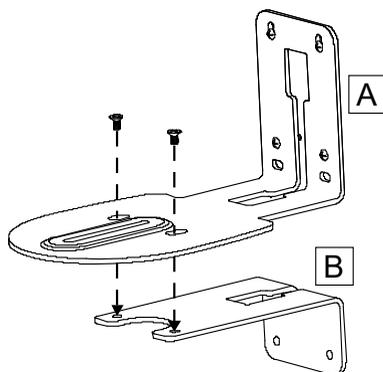
4. After assembling the L-mount brackets, use the screws (not included) to secure the lower part of L-mount brackets on the wall.
