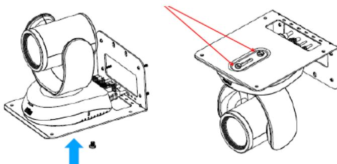
5. Find suitable screws to fix the camera mount to the ceiling.
