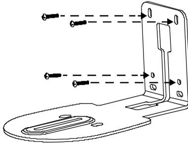
3. Then, assemble the L-mount brackets **A** + **B** with screws (included in package).
