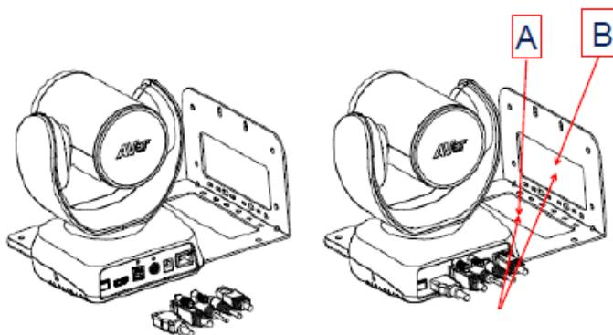
4. Turn the camera to face the front side. Install the second screw and tighten both screws.
